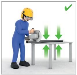
Secure the workpiece – Both hands on the machine
